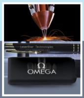
The laser engraving is a process fully controlled by computer, where the laser beam physically removes the surface of the material to expose desired design. At Dot Laser it can be done on a various materials such as wood, plastic, leather, glass, coated metal, anodised aluminium and many more. This is the most common option for people who want something personalised or customised from simple initials, names etc to creative fine art design.
